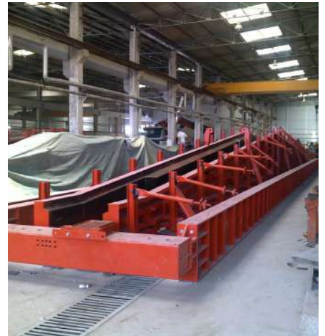
Uşak / TÜRKİYE Roof Truss Mould
