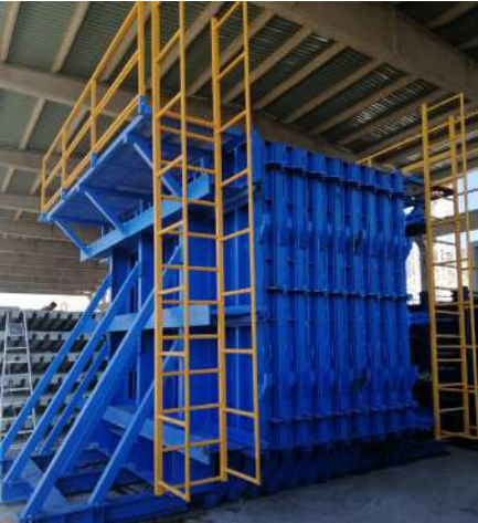
Dohuk / IRAQ Vertical Wall Mould (8 Batteries)
