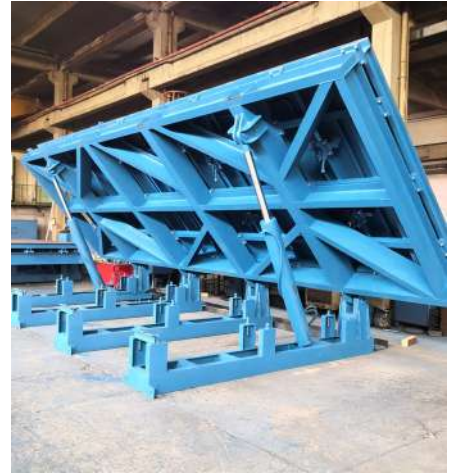
Tashkent / OZBEKSTAN Tilt - Up Table Wall Mould
